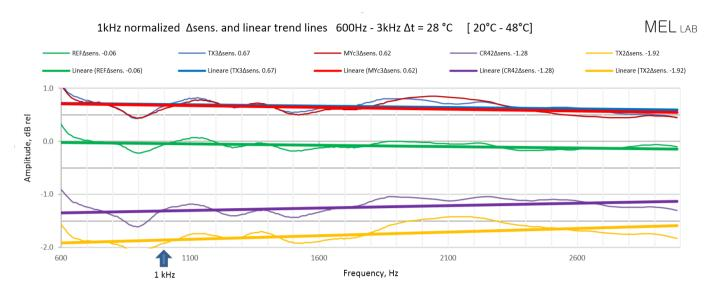
Fig. 7 All the curves representing the net difference,  $\Delta$  sens. and linear trend lines
