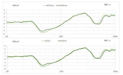
Fig. 5 The reference microphone curves at 20°C and 48°C before and after normalization
