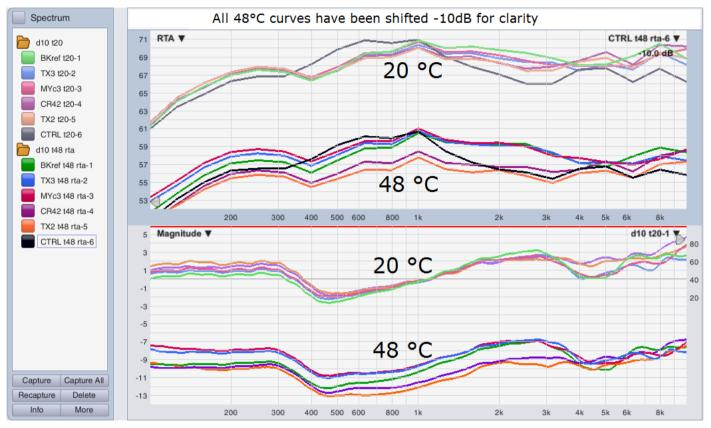
Fig. 3 1/3 ott spectra and T.F. responses of the microphones at 20°C and 48°C as taken
