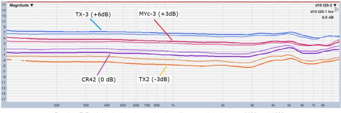
Fig. 4 T.F. of the 4 microphones Vs. the reference microphone at 20°C and 48°C
