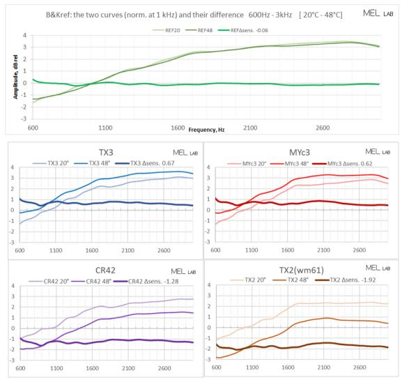
Fig. 6 All microphones curves at 20°C and 48°C and their difference (Δsens.)
