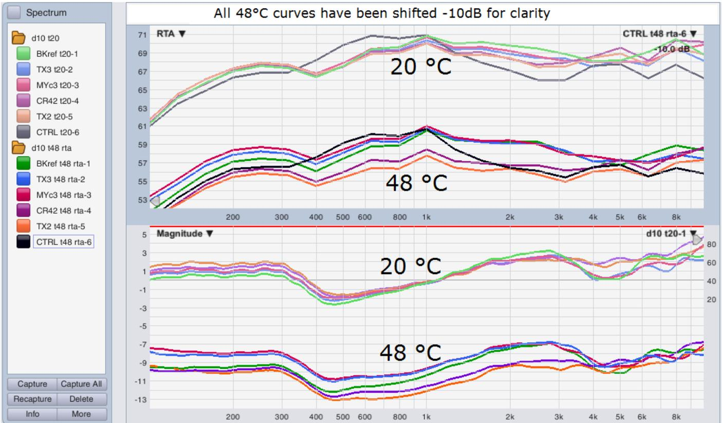
Fig. 3 1/3 ott spectra and T.F. responses of the microphones at 20°C and 48°C as taken
