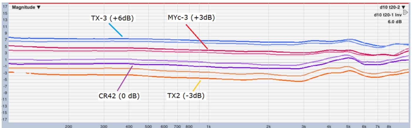
Fig. 4 T.F. of the 4 microphones Vs. the reference microphone at 20°C and 48°C
