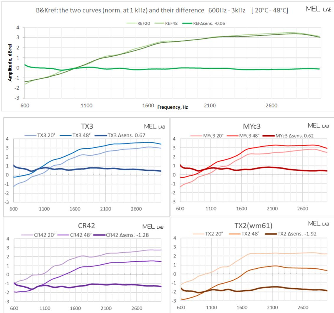
Fig. 6 All microphones curves at 20°C and 48°C and their difference ( $\Delta$ sens.)
