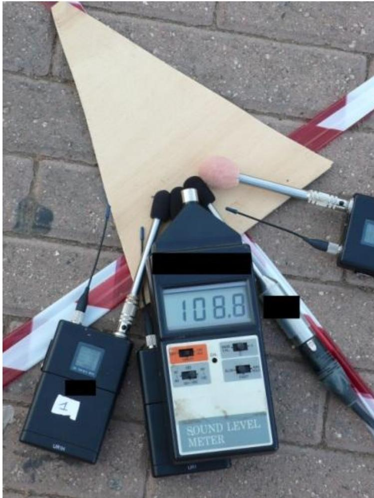
*Calibration of three wireless microphones (the pink one is “female”!) and one reference wired microphone with the sound level meter*
