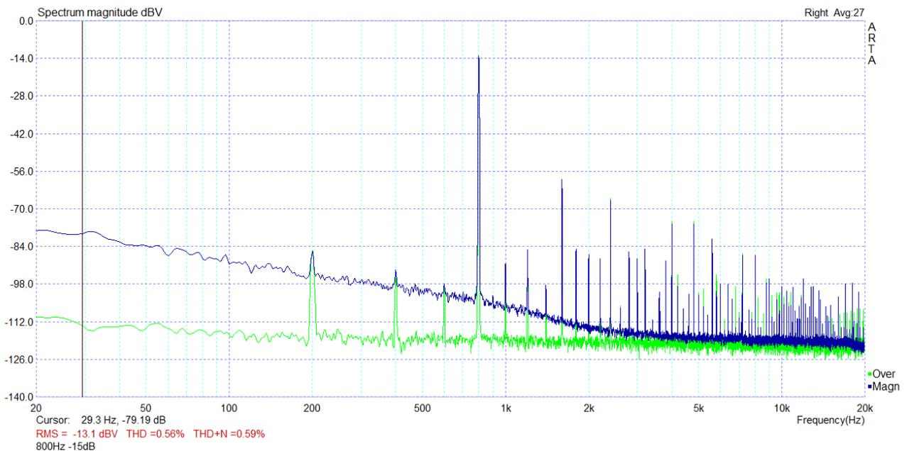
The frequency response "recommends" using the system from 50 Hz to 15 kHz. Distortion and noise do not seem to be a problem and compression phenomena can be avoided by properly adjusting the transmitter gain. In short, the system can be profitably used within certain limits, which are not serious at all.
