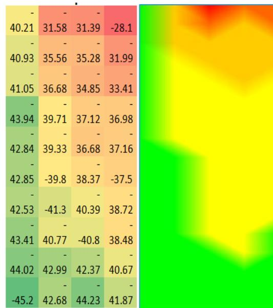
*[Numbers shown in the measurement matrix indicate the software/soundcard full-scale dBV level. They will then be normalized according to the calibration carried out on site.]*
